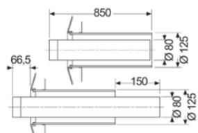
Terminal horizontal  $\varnothing 80/125$ mm
