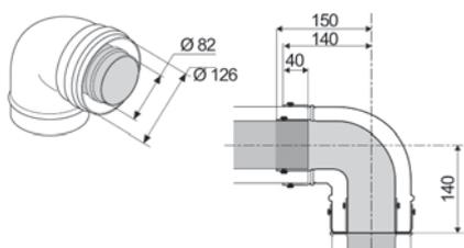
Codo  $90^\circ \varnothing 80/125$ mm
